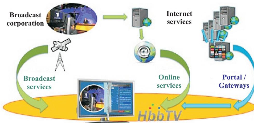
HbbTV doesn't depend on a particular broadcast link or on a particular IP link – it'll work with either [40]
