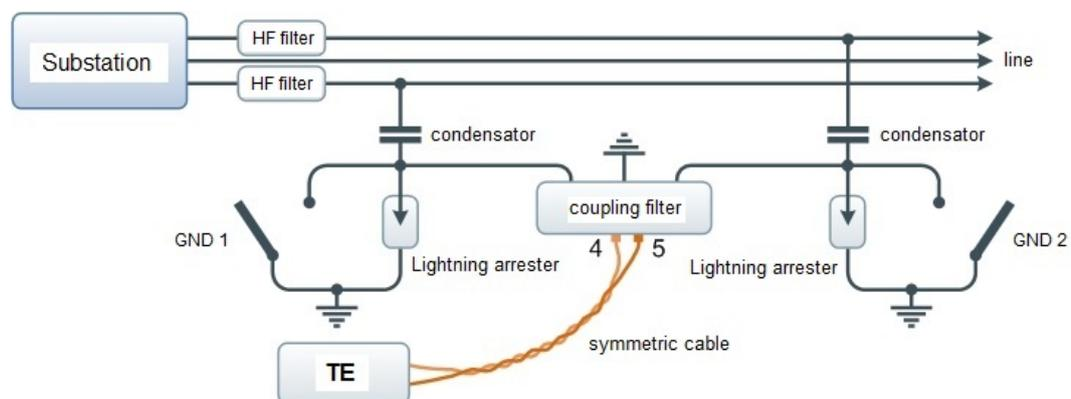
Schematic arrangement of most widely used interphase capacitive coupling high-frequency devices to high-voltage power lines.
