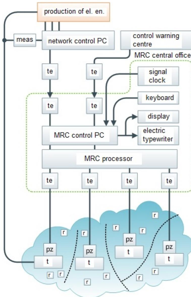
General arrangement of a modern MRC; te – transmission equipment, t – local MRC transmitter, r – MRC receiver.
