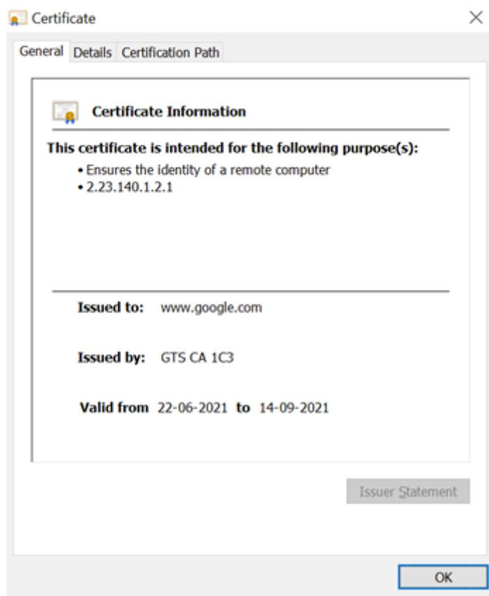
Fig. 33. Example of a digital certificate in Microsoft Windows.
