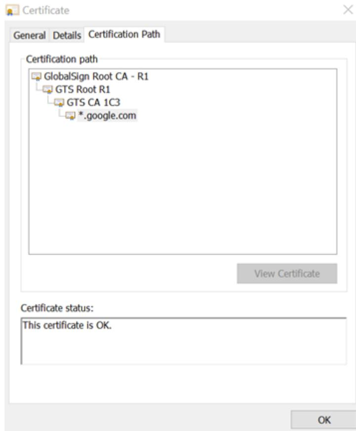
Fig. 35. Example of a Chain of Trust.
