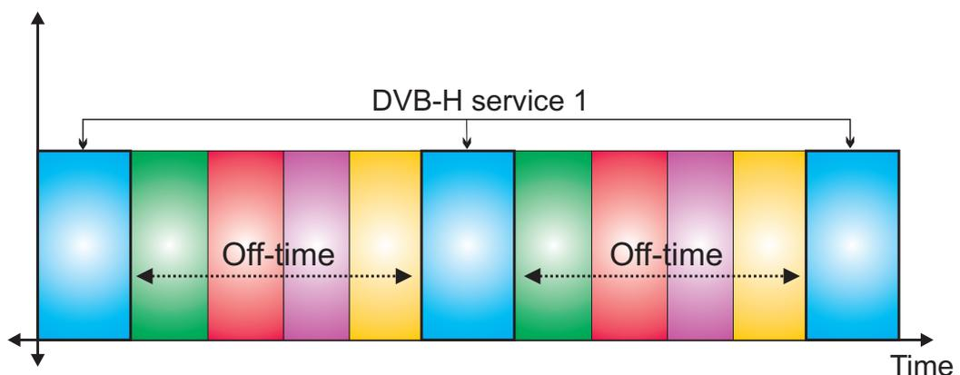
Fig. 8 - Time slicing principle
