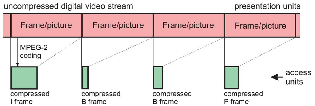
Fig. 3 - Coding by MPEG-2 coder
