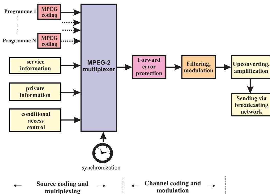
Fig. 6 - Block diagram of DVB transmitter
