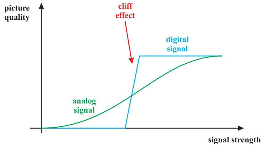
Fig. 2 - Digital television – how picture quality depends on signal strength
