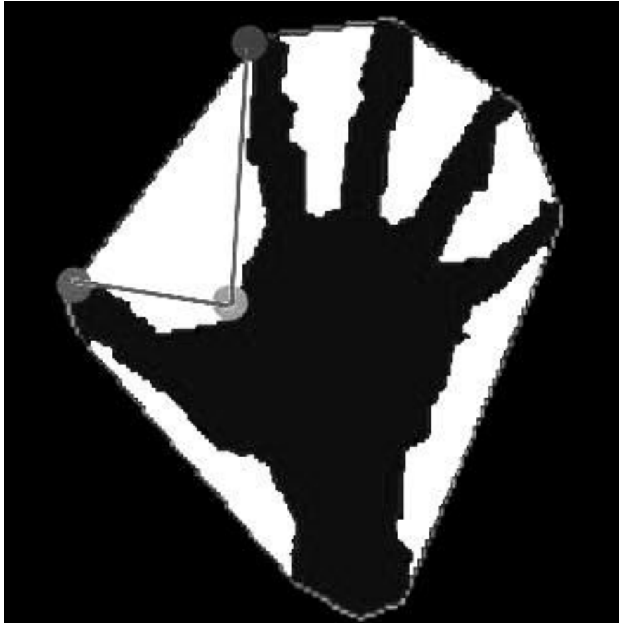
Fig. 4.4 – Marked areas are convexity defects and three points: start point (left), deepest point (bottom) and end point (top)
