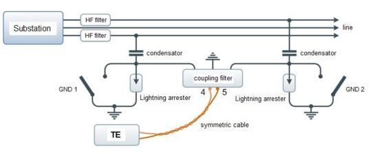
Schematic arrangement of most widely used interphase capacitive coupling high-frequency devices to high-voltage power lines.
