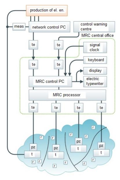
General arrangement of a modern MRC; te – transmission equipment, t – local MRC transmitter, r – MRC receiver.
