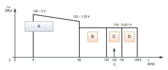
Frequency bands and limit values of the output voltage.
